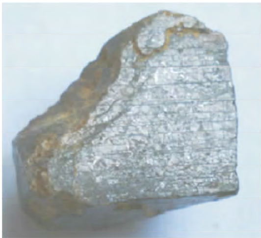
图 3 蓝宝石样品表面的聚片双晶纹 Fig. 3 Polysynthetic twins striation of surface of sapphire sample
